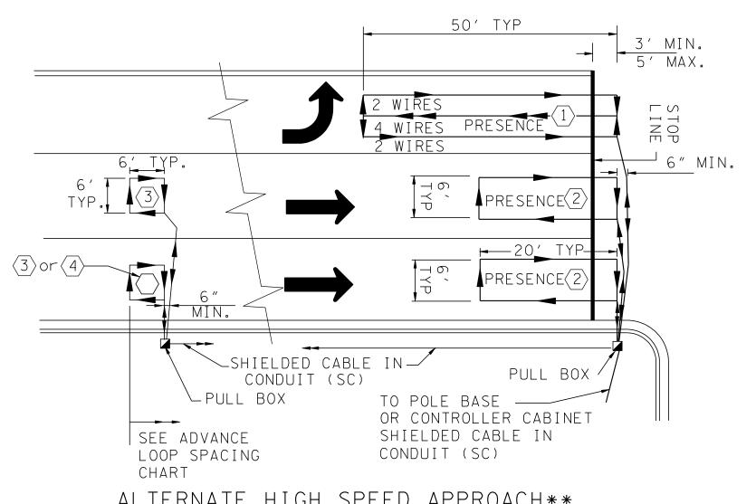
ALTERNATE HIGH SPEED APPROACH\*\* \*\* FOR USE WHEN PRESENCE DETECTION IS REQUIRED
